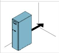
11. To secure the UPS cabinet in position, lower the leveling feet until the cabinet is not resting on the casters and the cabinet is level
