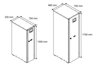
Figure 9. 93PS 8-40 kW UPS dimensions
