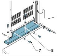
NOTE: After you have removed the shipping brackets, move the unit immediately away from the pallet.
