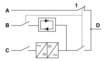
Figure 34. Maintenance bypass mode
