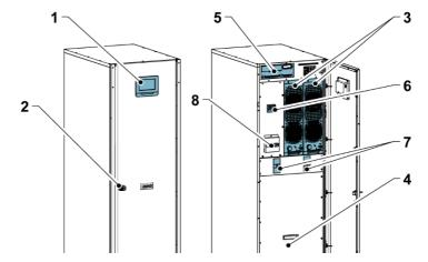
Figure 3. Looking inside the Eaton 93PS UPS 30-40 kW
