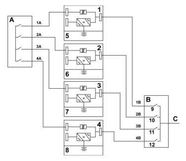
Figure 18. Principle of paralleled UPS systems
