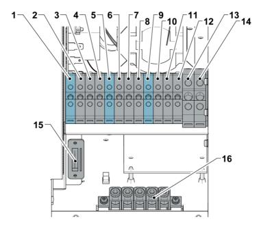
Figure 10. 93PS UPS 8-20 kW power cable terminals
