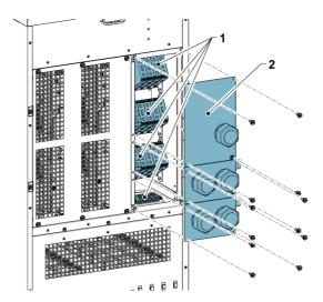
Figure 13. 93PS UPS 30-40 kW gland plate and connector locations
