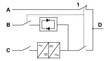
Figure 35. Maintenance bypass mode
