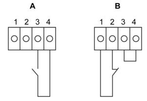
Figure 16. Connections of the EPO switch
