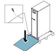
5. If the leveling feet are not fully retracted, turn them until they are retracted.
