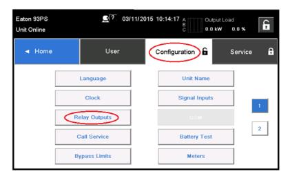
Figure 28. Selecting Relay Outputs in the Configurations screen
