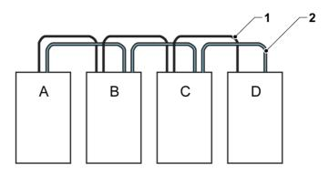
Figure 19. Simplified CAN and Pull-Chain wiring for parallel UPS system
