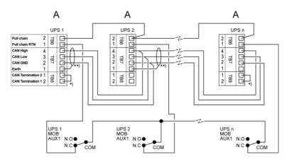
Figure 20. CAN and Pull-Chain wiring for parallel UPS with MOBs
