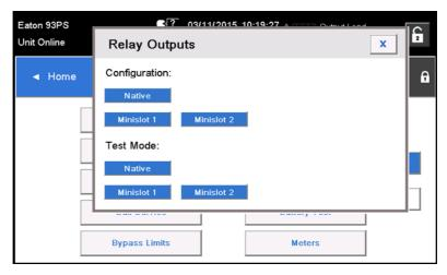
Figure 29. Options for relay outputs configuration
