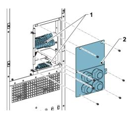
Figure 12. 93PS UPS 8-20 kW gland plate and connector locations
