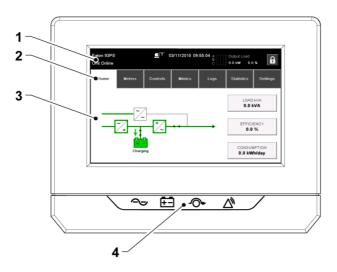
Figure 32. Parts of the display
